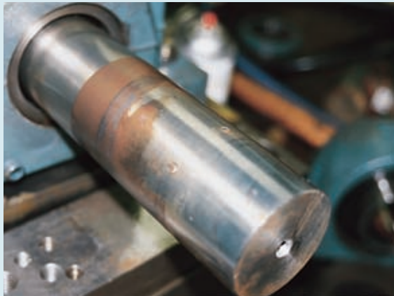
Typical Fretting corrosion and shaft damage with Setscrew Bearing
